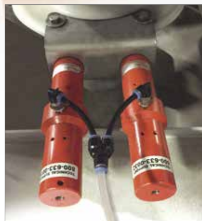
Vibrators used in tandem. All pneumatic piston vibrators require lubricated air for proper operation and long life. Low draw units like these 70-1's can share an air line and still run effectively.
