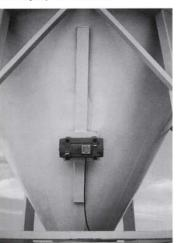
To select the proper size vibrator, calculate the total weight of the material in the sloping part of the silo.
