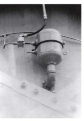
SOLUTION: One VIBCO Model ABS-2 Air Cannon was installed as shown in the photos, manually pushbutton operated from a control panel. With a few initial "blasts" a lot of "old cement" was cleaned out, and now cement flows on command every time. Air consumption has been cut to a fraction of what was used
