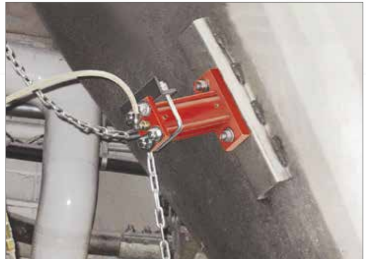
The LI Piston is used when a single impact is needed. Force and frequency adjustable by use of air pressure regulator and field adjustable timer.
