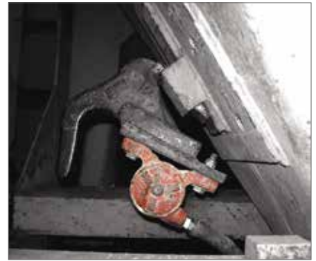
UWF-1 Female Bracket allows multiple hoppers to use one vibrator as needed.
