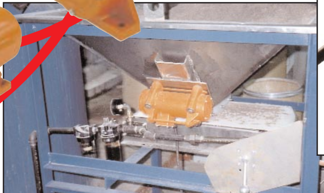
• SCR-200 keeps material flowing evenly to belt conveyor
