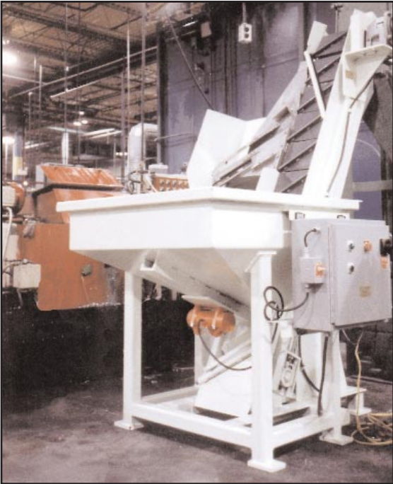
• Parts in dump hopper were interlocking. An SCR-100 on hopper separated them
